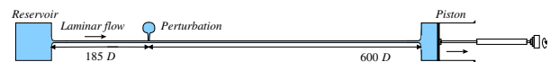
FIG. 1 (color online). Schematic diagram of the pipe flow facility (drawn to scale). The piston moves at a controlled speed and the fluid is pulled through the pipe at constant mass flux. The usable experimental run time is \approx 30 min.
