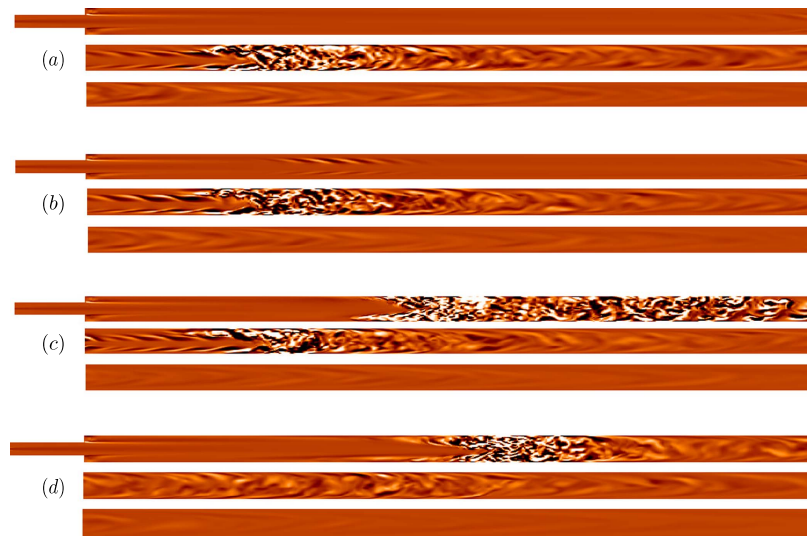
Figure 4. x - z cross sections of streamwise vorticity contour plot for Re = 2000 with \delta = 0.1 at (a) t = 1000 , (b) t = 1025 , (c) t = 1050 and (d) t = 1100 . Each triad represents the full pipe length, truncated at every 50d for simple visualisation purpose. Here black and white corresponds to the maximum and minimum of vorticity and orange (grey) represents zero vorticity.
